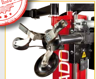
MULTI-FUNCTIONAL REVOLVER TOOL 4 TOOLS - 3 POSITIONS - AUTOMATIC ROTATION
