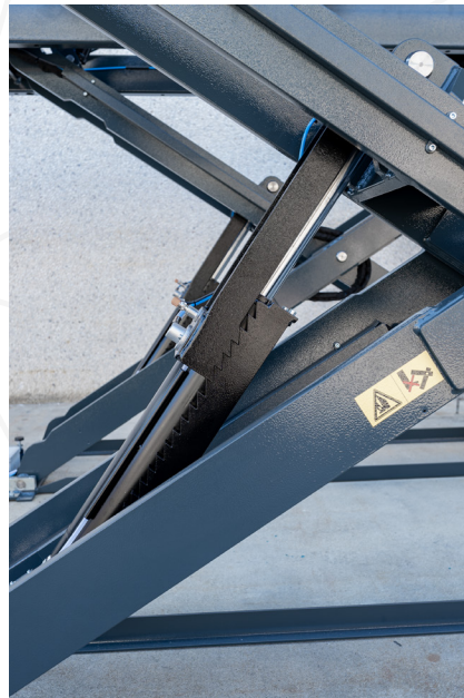
MECHANICAL SAFETY rack on cylinder with cold galvanizing treatment
