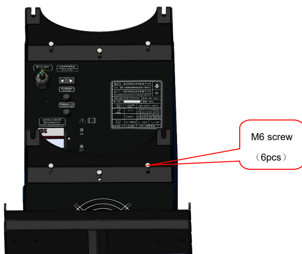
( FIG 6 Gas bottle U-Style bracket installation drawing )
